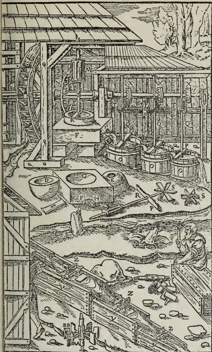
A—WATER-WHEEL. B—AXLE. C—STAMP. D—HOPPER IN THE UPPER MILLSTONE. E—OPENING PASSING THROUGH THE CENTRE. F—LOWER MILLSTONE. G—ITS ROUND DEPRESSION. H—ITS OUTLET. I—IRON AXLE. K—ITS CROSSPIECE. L—BEAM. M—DRUM OF RUNDLES ON THE IRON AXLE. N—TOOTHED DRUM OF MAIN AXLE. O—TUBS. P—THE SMALL PLANKS. Q—SMALL UPRIGHT AXLES. R—ENLARGED PART OF ONE. S—THEIR PADDLES. T—THEIR DRUMS WHICH ARE MADE OF RUNDLES. V—SMALL HORIZONTAL AXLES SET INTO THE END OF THE MAIN AXLE. X—ITS TOOTHED DRUMS. Y—THREE SLUICES. Z—THEIR SMALL AXLES. AA—SPOKES. BB—PADDLES.
